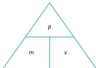
**Figure 7.32** The momentum triangle. Cover the quantity you want to calculate and the other two quantities will form the formula.
