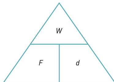
**Figure 7.36** The work triangle. Cover the quantity you want to calculate and the other two quantities will form the formula.
