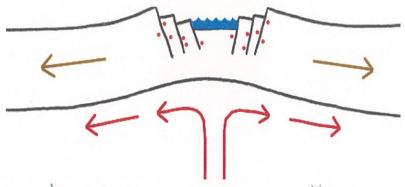
As the plate moves apart, the blocks slide <u>down</u> the <u>Fault plane</u>, pulled down by gravity.
