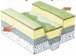
Normal Faults occur typically in <u>kift</u> <u>valleys</u> where continents are being pulled apart due to an upwelling <u>convection</u> current.
