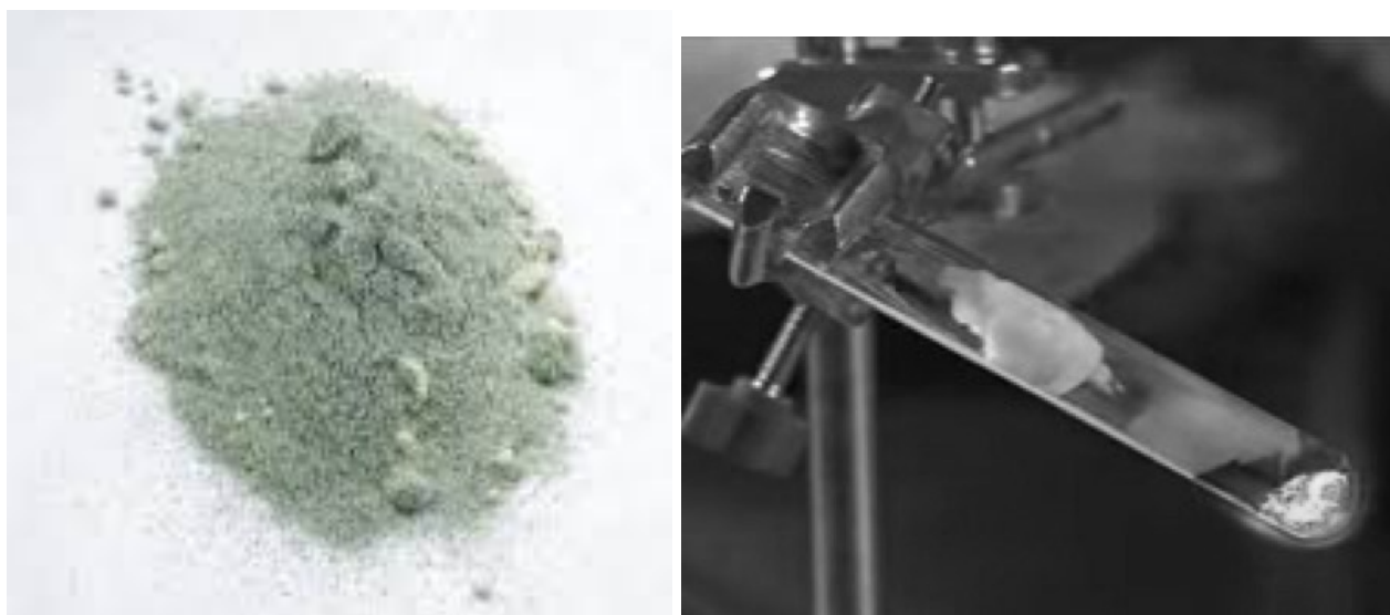
Figure 3 Mixture of iron and sulphur (left) and Iron and sulphur heating (right)
