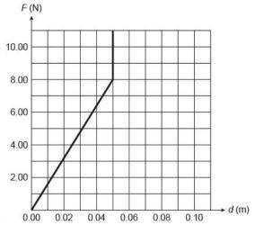
The energy stored in a spring can be determined by calculating the area underneath its force (N) against extension (m) graph.
