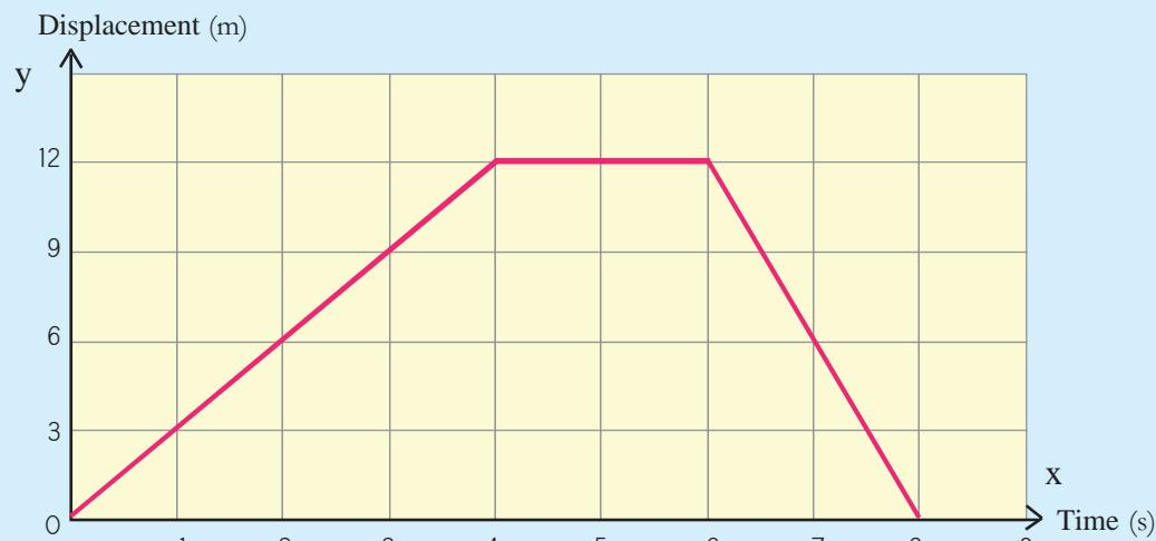
Fig : 1.9 ▲ Displacement - time graph
