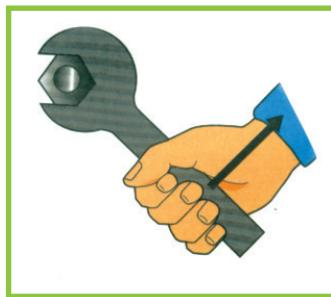
Fig : 1.35 Moment of force applied by a spanner
