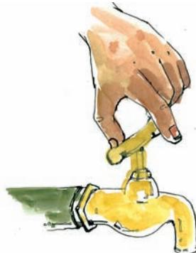
Fig : 1.37 ↑ Couple of forces applied on a tap
