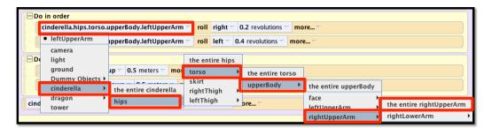
We want the new block of code to refer to the right arm. Click on the arrow next to leftUpperArm in the first roll method in the block and select Cinderella, hips, torso, upperBody, rightUpperArm, the entire rightUpperArm.
